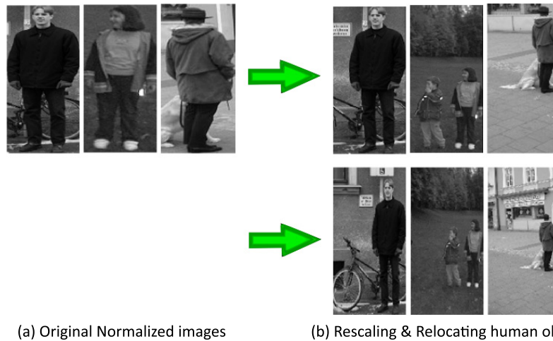
Fig. 5 Examples of the human images. The left shows those in the original INRIA data set provided by Dalal 100 \times 200 [pixels 2 ] [11]. The right top shows those of the dataset 1, which is re-cropped into 180 \times 400 [pixels 2 ] and re-scaled into 100 \times 200 [pixels 2 ]. The right bottom shows those of the dataset 2, which is re-cropped into 300 \times 600 [pixels 2 ] and re-scaled into 100 \times 200 [pixels 2 ].
