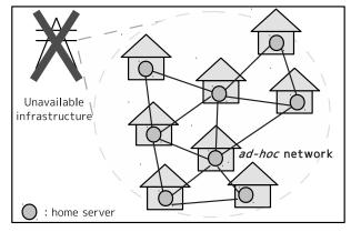
Fig. 2 Construction of Ad-hoc networks
