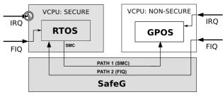
Fig. 3 Execution paths of the SafeG monitor.
