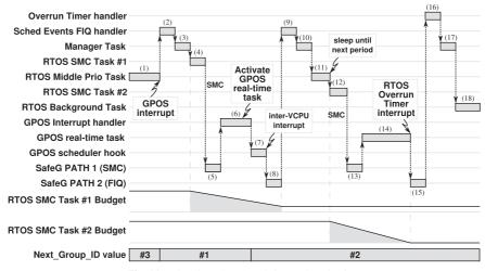
Fig. 11 Timeline: GPOS real-time task activation.
