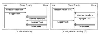
Fig. 15 Execution priority levels for the use case example.
