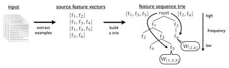
Fig. 2 Feature sequence trie and completion of prefix feature vector weights.
