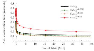
**Fig. 7** Average classification time per sentence plotted against size of fstrie in dependency parsing: svM<sub>3</sub>.
