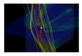
Figure 1. The magnetic field lines tracing in the region from the subsolar point to  $\pm 5 \mathrm{Re}$  in the dawn-dusk directions. These lines reconnect with the geomagnetic field at the dayside magnetopause.
