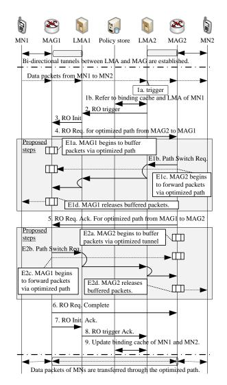
Fig. 3 Route optimization procedure with optimized path switching. Signaling messages are indicated by a solid line while data packets are indicated by a dotted line. The procedure regarding the optimized path switching is enclosed by boxes.
