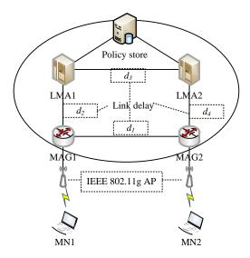
Fig. 4 Network topology of experimental testbed.
