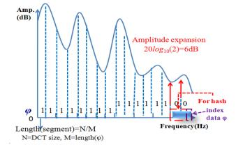
$\boxtimes$  5 Amplitude expansion: highest frequency region is reserved to embed index data  $\vec{\varphi}$ , with length equals M = 16. The embedding region is divided into two parts: hash data (length=160 bits), and index table for hiding  $\vec{\varphi}$ (length = M);
