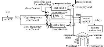
**3** Structure of extraction and verification phases
