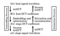
$\blacksquare$  4 Signal representations. t is discrete time;  $0 < t \le N$ . i is discrete frequency;  $0 < i \le N$ .
