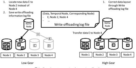
$\boxtimes 2$  Data layout correction from write offloading
