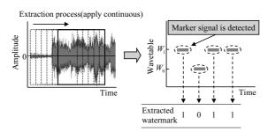
Figure 3: Processing flow of extraction
