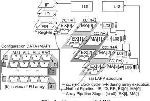
Fig. 1 Structure of LAPP.
