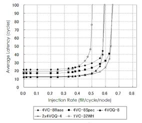
Fig. 9 Network latencies of routers with 8-flit buffer (4VC-8Base = four 8-flit VCs/port Baseline; 4VC-8Spec = four 8-flit VCs/port LA+Spec; 4VOQ-8 = four 8-flit VOQs/port; 2x4VOQ-4 = eight 4-flit VOQs/port; 1VC-32WH = one 32-flit VC/port).
