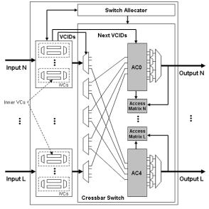
Fig. 6 Multiple VOQ architecture.
