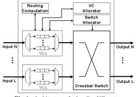
Fig. 1 Architecture of a baseline VC router.
