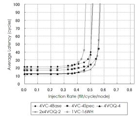
Fig. 8 Network latencies of routers with 4-flit buffer (4VC-4Base = four 4-flit VCs/port Baseline; 4VC-4Spec = four 4-flit VCs/port LA+Spec; 4VOQ-4 = four 4-flit VOQs/port; 2x4VOQ-2 = eight 2-flit VOQs/port; 1VC-16WH = one 16-flit VC/port).
