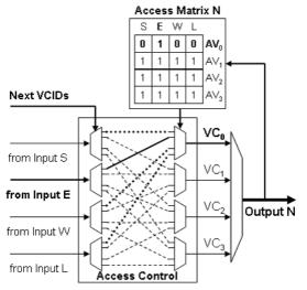
Fig. 5 Access control logic for output VCs.
