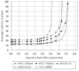
Fig. 10 Network latencies of routers with 16-flit buffer (4VC-16Base = four 16-flit VCs/port Baseline; 4VC-16Spec = four 16-flit VCs/port LA+Spec; 4VOQ-16 = four 16-flit VOQs/port; 2x4VOQ-8 = eight 8-flit VOQs/port; 1VC-64WH = one 64-flit VC/port).
