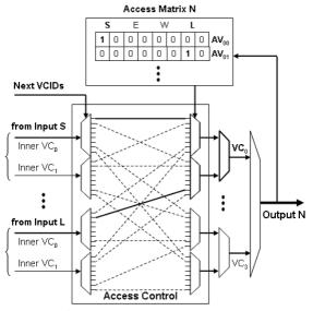
Fig. 7 Access control logic for output inner VCs.
