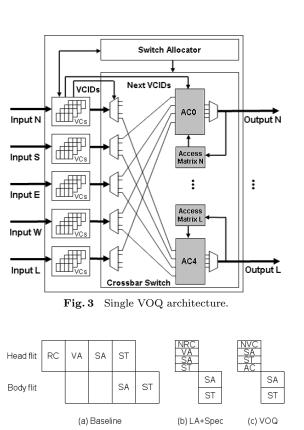
Fig. 4 Comparison of pipeline stages of a packet transfer between (a) baseline router, (b) look-ahead speculative (LA+Spec) router, and (c) proposed VOQ router.
