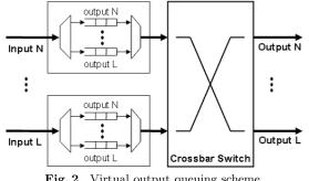
Fig. 2 Virtual output queuing scheme.
