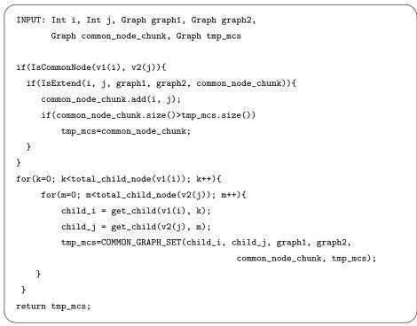
Fig. 8 COMMON\_GRAPH\_SET function for connected common subgraph.
