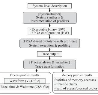
Fig. 2 Tool flow of the profilers supported by SystemBuilder.
