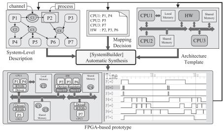
Fig. 1 Design flow of SystemBuilder.
