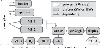
**Fig. 10** Functional structure of the MPEG4 decoder.
