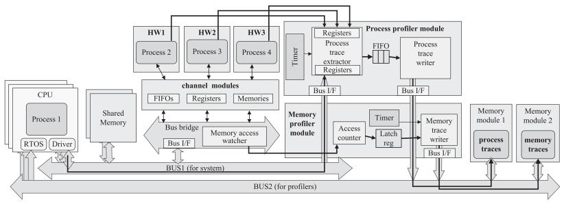
Fig. 3 Overall structure of the process profiler and the memory profiler.
