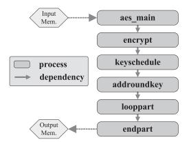
Fig. 6 Functional structure of the AES encryption system.
