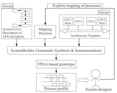
Fig. 7 Design space exploration scenario of AES design.
