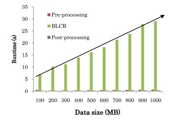
Figure 2 Relation between data size and checkpoint overhead in our CUDA checkpointer
