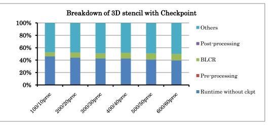
Figure 4 Breakdown of 3D stencil with checkpoint
