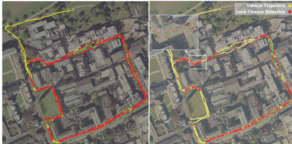
Fig. 3. Result of City Centre dataset analysis. Yellow dots represent the vehicle's trajectory. Red dots represent the location with loop-closure detection. Left figure shows the aerial result of our system. Right figure shows the aerial result of FAB-MAP [2].
