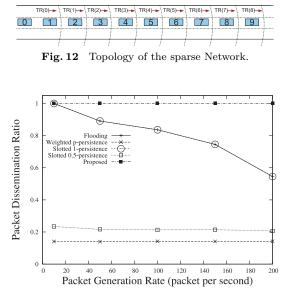
Fig. 13 Packet delivery ratio for various packet generation rate.
