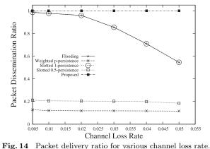
persistence and slotted 1-persistence, they behave poor performance in a sparse network because of probabilistic broadcasting. However, thanks to retransmission mechanism, the proposed protocol can achieve one hundred percent delivery ratio.
