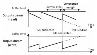
Fig. 2 I/O request deadline relation to a stream buffer state.
