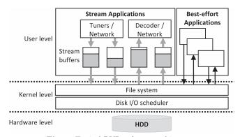
Fig. 1 Typical DVR software architecture.
