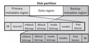
Fig. 5 Disk partition format with the A/V file system.
