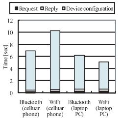
Fig. 8 Time required to complete the network composition procedures.
