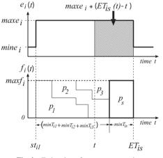
Fig. 4 Estimation of power consumption.
