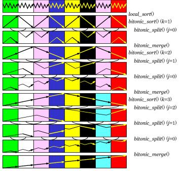
Fig. 3 Progress of bitonic sort with 8 processes.
