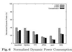
extra leakage induced by a second 64bits register. With our iTLB leakage control mechanism, average 50% leakage power and 70% dynamic power can be reduced
