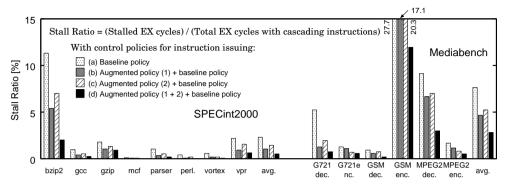
Fig. 6 Stall ratios on the single bypass network after applying different levels of conflict reduction policies in Section 3.2.
