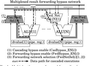
${\bf Fig. 4} \quad {\rm Multiplex \ the \ usage \ of \ normal \ forwarding \ by passes}.$
