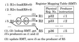
Fig. 2 An RMT implementation to trace the direct producer instruction, as well as the logical/physical register mapping.
