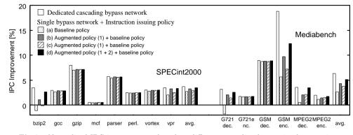
Fig. 7 Normalized IPC improvements based on different cascading bypass implementations.
