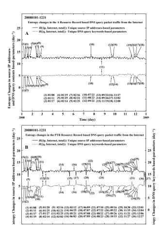
Figure 4. Entropy changes in the total A and PTR resource records (RRs) based DNS query request packet traffic from the Internet to the top domain DNS (tDNS) server through January 1st to December 31st, 2008. The solid and dotted lines show the unique source IP addresses and unique DNS query keywords based entropies, respectively (day<sup>-1</sup> unit).
