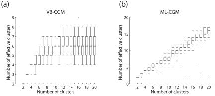
Fig. 3 The number of effective clusters in the CGM models. (a) Schematic plot of the number of effective clusters versus the number of all clusters by the VB-CGM. Note that the vertical axis represents discrete values. (b) Schematic plot of the number of effective clusters versus the number of all clusters by the ML-CGM.
