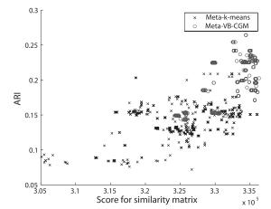
Fig. 4 Objective function of meta-cluster analysis and ARI. Scatter plot of the ARI versus the objective function (Eq. (10)), in the VB-CGM method (circles) and the k-means clustering (crosses).
