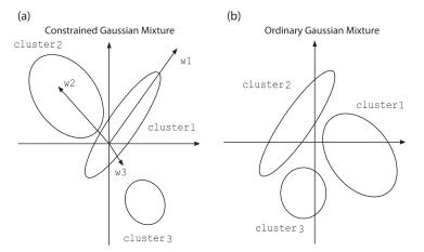
Fig. 1 CGM model and Gaussian mixture model. Conceptual illustration of (a) the proposed constrained Gaussian mixture (CGM) model and (b) the ordinary Gaussian mixture model. Ellipses represent covariances of clusters. The arrows in (a) represent the  $\boldsymbol{w}$  vectors of the clusters, which are constrained to go through the origin.
