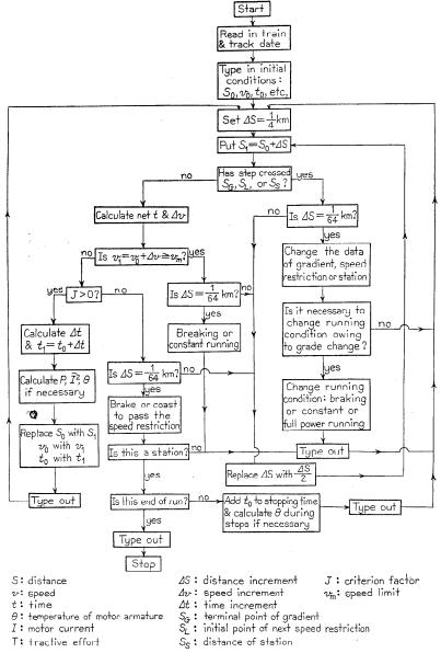
Fig. 1. Block scheme for train performance calculation
