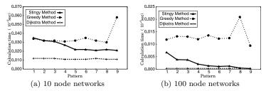
Fig. 4 Mean time to calculate the broadcast tree.
