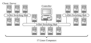
Fig. 9 Experimental setup for data replication protocols.
