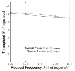
**Fig. 12** Average throughput for probabilistic TP using  $s_l = 2l + 3$ , h = 2, N = 15, p = 1.0, f = 0.5, and w = 1.
