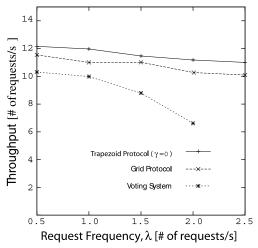
**Fig. 11** Average throughput on data replication protocols (  $N \approx 15$  and p = 1.0 ), TP:  $s_l = 2l + 3$ , h = 2, N = 15, f = 0.5, w = 1,  $\gamma = 0.0$  and grid protocol:  $4 \times 4$ , VS: N = 15, |RQ| = 8, |WQ| = 8.
