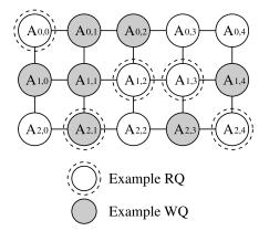
Fig. 1 Example of Grid Protocol with  $3 \times 5$  nodes. Examples of RQ and WQ are the set of nodes circled with dotted line and painted gray, respectively.
