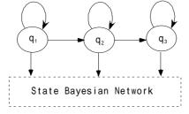
Figure 2: The hybrid HMM/BN model structure.
