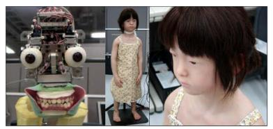
Fig. 1 The android *Replice R1* is a replica of a five-year-old Japanese girl. Her arms, neck, head, eyes, and eyelids are powered by DC motors fixed inside the robot. Her skin is made of silicone. In the photograph on the left, the android's skin, hair, and padding have been removed.
