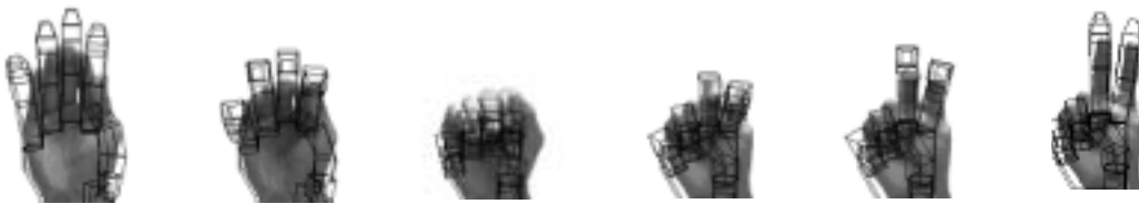
Fig. 6 Examples of behaviour of human hand and estimated joint angles.
