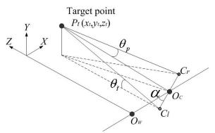
Fig.3 Control of parameters:  $(x_t, y_t, z_t)$  is the coordinate of the target point in the camera coordinate system
