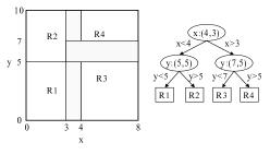
Fig. 1 Image of partitions (left) and its index structure (right)
