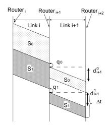
Figure 1: Packet Pair Model in FIFO
