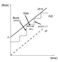
Figure 13: Packet Train Model in Token Bucket Model
