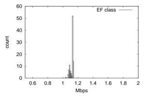
Figure 8: histogram of bps, packet size is 1450 bytes
