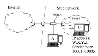
Figure 1: Traffic measurement points.
