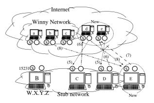
Figure 3: Procedures of our proposed identification method 2.
