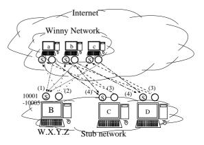
Figure 2: Procedures of our proposed identification method 1.
