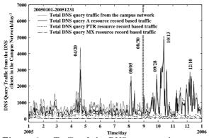
Figure 3. Traffic of the DNS query packet access from the outside of the campus network through January 1st to December 31st, 2005  $(day^{-1} unit)$ .
