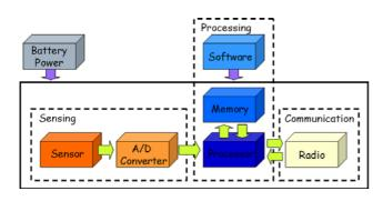
Figure 1 : Sensor Network Node Architecture
