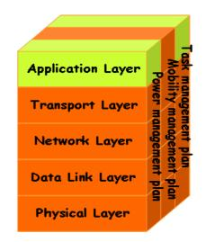
Figure 3 : Sensor Network Protocol Stack
