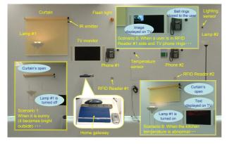
Fig. 5 Experimental system using Home Service Harmony
