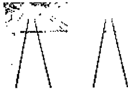
Fig. 7: Detected rails by pixel-valued methods (left) and finally output image of rails (right).
