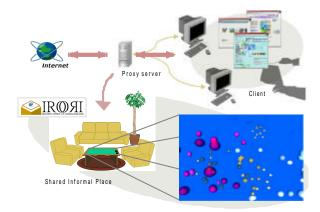
**Fig. 5.** Structure of IRORI system. Each vapor on the screen of horizontal PDP is linked to an URL that a client had accessed previously
