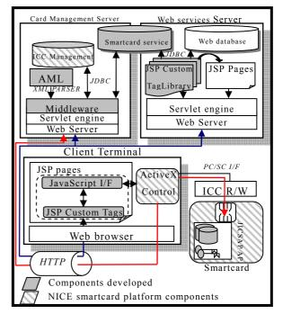
Figure 4. Prototype system overview
