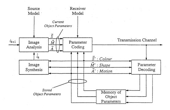
Fig. 1: Block diagram of an object-based analysis-synthesis coder [1]
