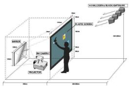
Figure 2. SenseWeb hardware setup: 150-inch screen, rear projection, camera with infrared (IR) filter and halogen lamps (as IR light source)
