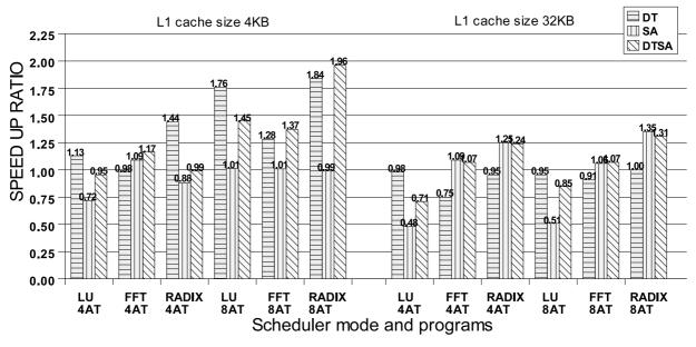
Figure 4. The speed up ratio by scheduler mode \*The speed up ratio of none scheduler mode is defined as 1.00 on each of benchmarks.
