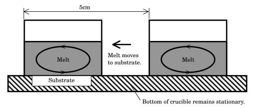
Fig.1 Movement of melt just before crystal grows
