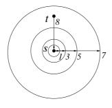
$\square$  1: Illustration of the doubling algorithm. Numbers represent transmission times, with the transmission range doubled by the sender s at each round until reaching the receiver t.
