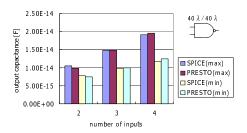
**Fig. 5** Output capacitance of a NAND gate at 100nm process.
