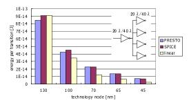
Fig. 4 Energy consumption of a FO4 inverter.
