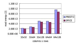
Fig. 6 SRAM read energy at 100nm process.
