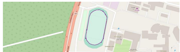
Fig. 11 5G Round 1: (188 samples) EKF error = 0.53% Pantai error= 1.60%.
