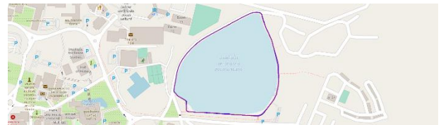
Fig. 8 5G Round 1: (618 samples) EKF error = 1.78% Pantai error= 5.18%.
