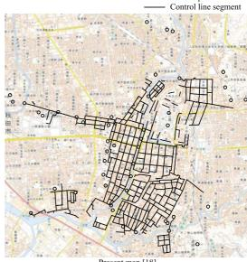
Fig. 5 Control points and control line segments used in geometric correction.
