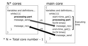
Fig. 5 Method of measuring the execution time
