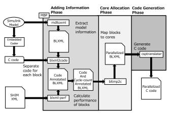
Fig. 3 System model of Model Based Parallelizer (MBP)
