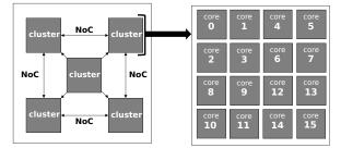
Fig. 2 Overview of Kalray MPPA3-80 Coolidge architecture
