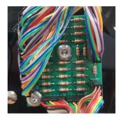
Fig. 7 Printed circuit board connected to 32 pressure sensors.
