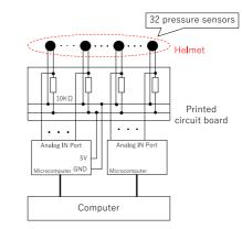
Fig. 2 Structure of device.
