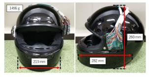
Fig. 9 Size of the prototype device.
